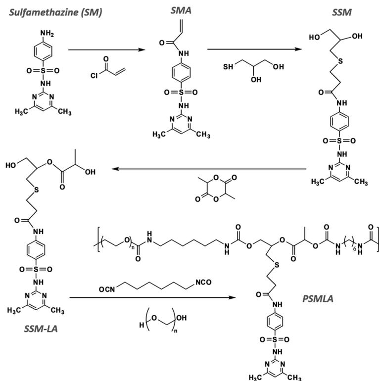
**Figure 1.** Schematic synthesis routes of SMA, SSM, SSM-LA monomers and PSMLA copolymer
